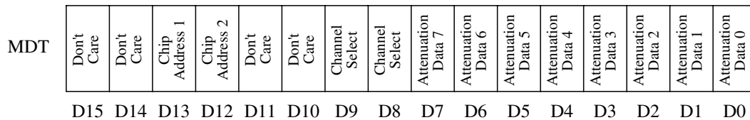
Figure 2. Microcontroller data format
